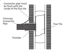
Make sure the connector pipe or thimble sleeve does not protrude into the flue liner, thereby restricting the area the smoke has to flow through. This bottle-neck will have a negative affect on the chimney system.
